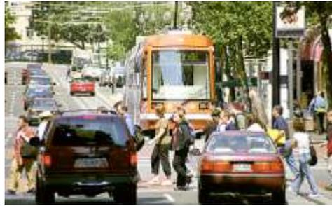
**Fit Within the Urban Environment.** Design tradeoffs were made to better fit the Portland Streetcar into the scale and traffic patterns of the neighborhoods through which it travels. Streetcar vehicles, manufactured in the Czech Republic, are 8 feet wide and 66 feet long. They run in mixed traffic and, except at stops, accommodate existing curbside parking and loading. Streetcar stops occur every few blocks and shelters are smaller to fit within the neighborhood’s architecture.
